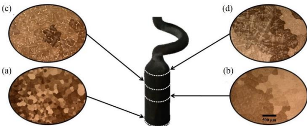
Figure 5. Microstructural images with 50 times magnification of cross-sections of the starter block at distances a)0, b)14, c)21 and d)29 mm from the chill plate.
