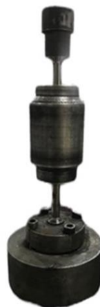
Figure 3. shows the double action die used in the compression process of the iron oxide powder and NaCl space holder mixture.
